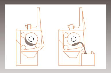
Empire's Continuous-Belt Blasters unload parts with the push of a button. Once processing is complete, the operator opens the door, pushes the "reverse" button and the barrel rotates in the opposite direction to feed work pieces into a post-processing bin.
